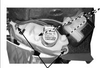
Screws of the horizontal vane motor unit
